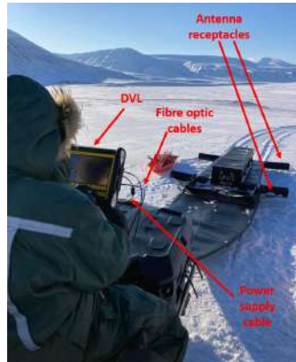
(b) pulseEKKO 100 MHz on black sledge. Image credit: J. Jonas, UNIS student
