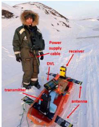
(a) pulseEKKO 100 MHz on orange sledge. Image credit: M. Richter, UNIS student
