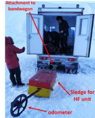
(c) pulseEKKO 900 MHz on HF sledge. Image credit: J. Jonas, UNIS student
