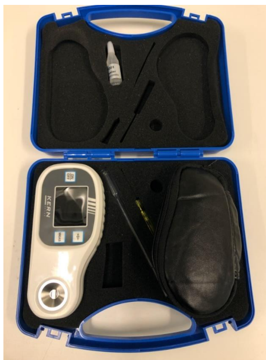
Figure 19 Digital refractometer used for measuring the concentration
