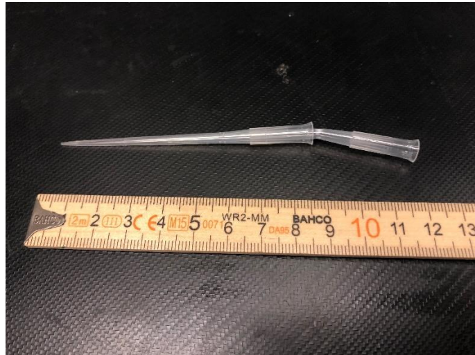
Figure 12 Modified pipette tips used in tests
