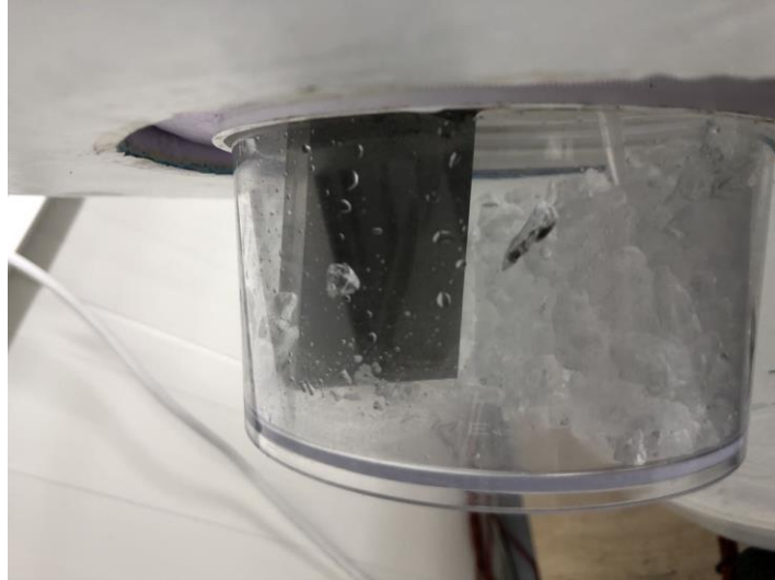
Figure 14 Meltwater stick on the wall of the plastic reactor separately (30 mins, NaCl)
