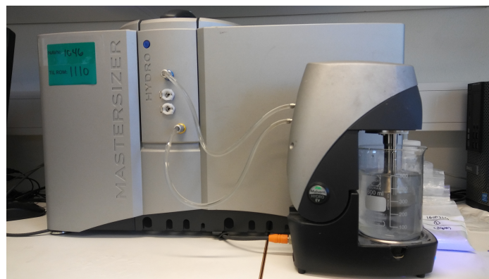
Figure 3.7: Malvern Mastersizer 3000 and propellor used for laser diffraction at NTNU
