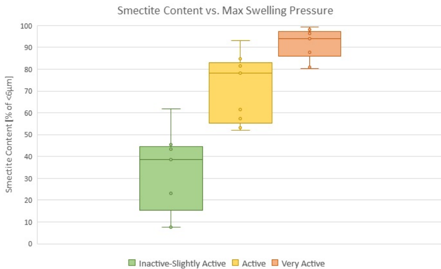
Figure 4.3: Smectite content in the <6µm fraction resulting in various levels of swelling pressure activity
