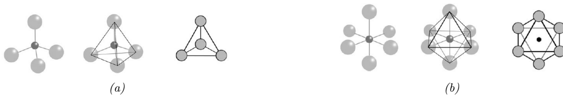
Figure 2.13: Ball-and-stick models and polyhedral models for tetrahedra (a) and octahedra (b) molecular structures [4]
